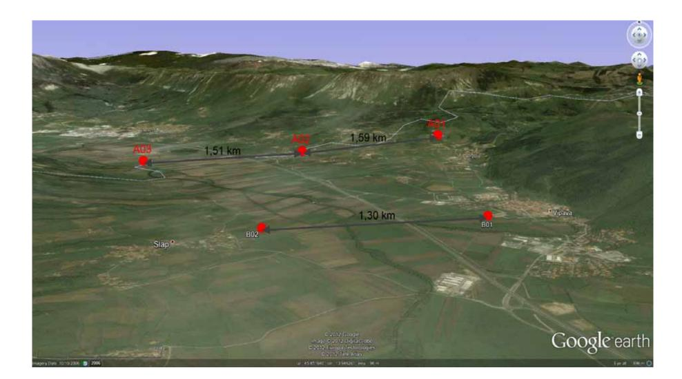
Locations of five new measurement sites in the Vipava valley along two lines. These are first observations of bora in the direction perpendicular to the Vipava valley orography. Wind gauges were mounted approximately 4 m above the ground.
