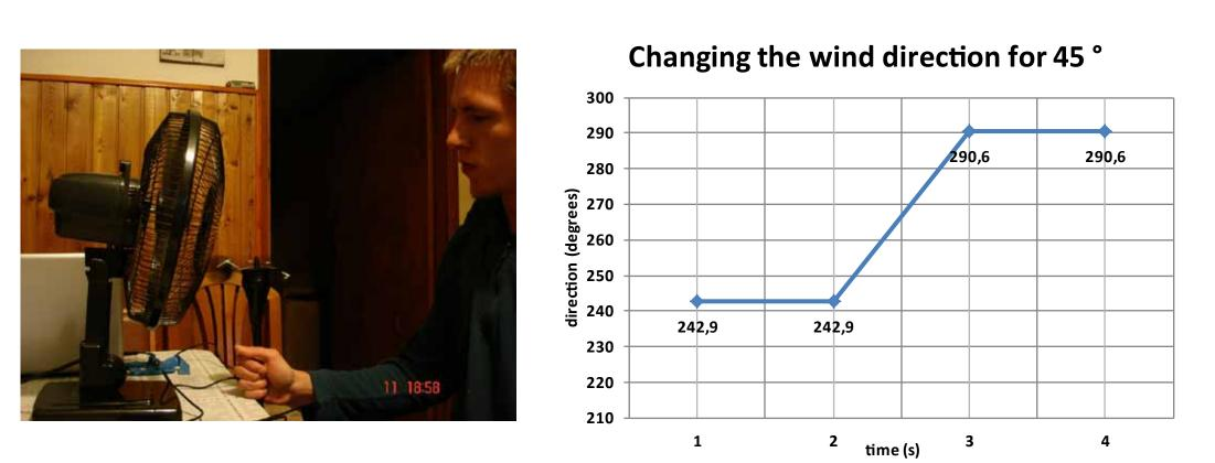
The response time, which we determined for HOBO wind gauges used in the project, was about 5 - 8 seconds, depending on the wind speed.
