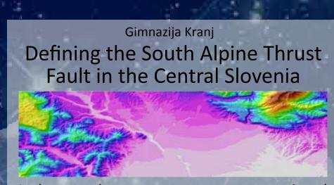
In the research paper we present a new tectonic and structural interpretation of the South Alpine Thrust Fault in the Central Slovenia, between the Kropa village and Kamnik. The new interpretation is based: (1) on geologic field work and mapping, (2) on the analysis of the digital terrain model of Slovenia and (3) on the numerous microtectonic studies and interpolation of the paleostress fields in the geological past of the region
