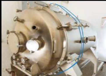
Thermal-vacuum chamber and satellite testing facilities
